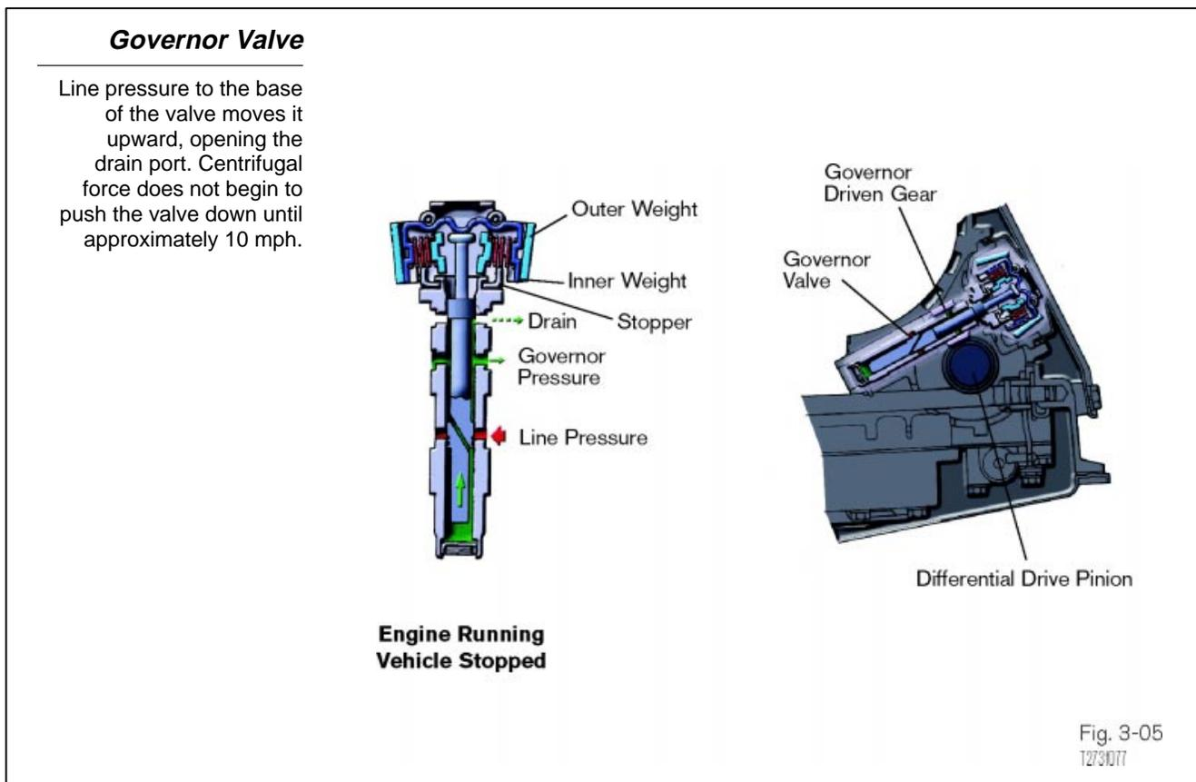
As vehicle speed increases, the weights move outward and the governor valve is pushed down by the lever of the inner weights. The governor valve position is balanced between centrifugal force acting on the lever at the top of the valve and governor pressure at the base of the valve.
