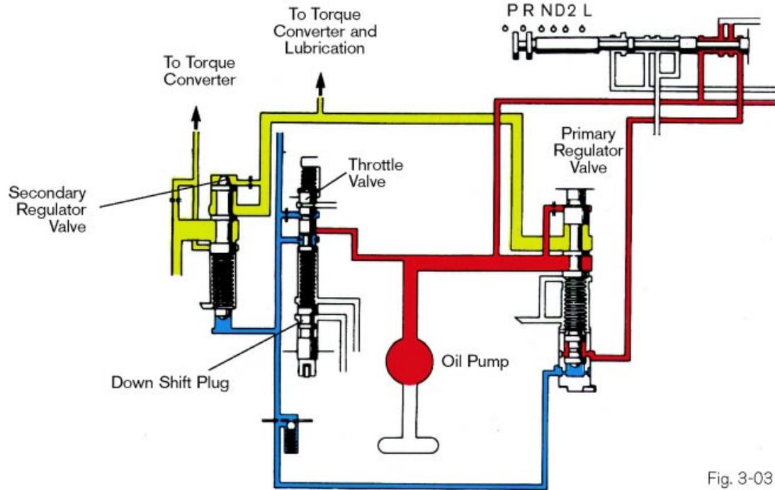
Line pressure is also increased when reverse gear is selected. Line pressure from the manual valve is directed to the bottom of the valve pushing it upward, increasing line pressure by as much as 50%.
